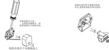
(3) Check fuse specifications and replace the fuse to the same specifications as the fuse listed in 1.7.1;
