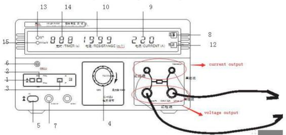
1.before turning on the power supply, instrument panel: test/preset  $\Omega$  1,200 m / 600 m  $\Omega$  2, alarm 3, three buttons keep up,The "current" adjusting knob 4 is set counterclockwise to 0.
